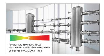
Air volume standard calibration system Air volume :  $1 \text{ m}^3/\text{h} \dots 1000 \text{ m}^3/\text{h}$
